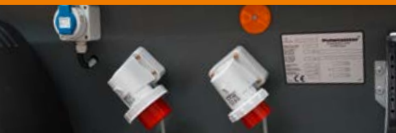
Standard 32 A socket and 16 A socket with optional additional drive
